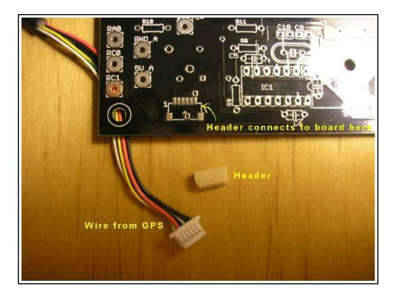
In this picture the header shown is oriented with the pins facing the bottom of the image, while it needs to be soldered into place with the pins facing the top of the image. Make sure the six pins on the header line up with the six pads, and the two support pins on the front of the header line up with the two support pads on the PCB (closest to the edge of the PCB).
